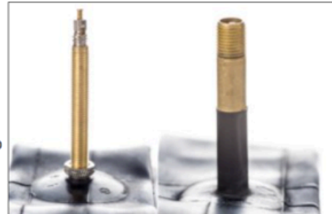
There are two types of valves for bike tubes: Presta (left) and Schrader (right). Presta valves are typically found on tubes for higher pressure tires. They require a compatible pump, or an adapter.
